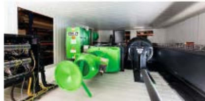
Hoists also rope hoists and crane control are built in the housing. A heating system ensures that the temperature inside the housing never drops below -20 °C. The system's explosion protection is thus guaranteed even at sub-zero temperatures.
