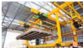
The wire rope hoist can be coupled for further operation, for example to lift the position and to change the force. Labels are visible both to be seen on outside the gantry crane.
