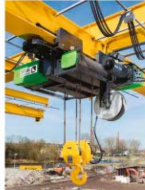
The 20-ton wire rope hoist is frequency-controlled and has a high FE30 1.5 classification with working loads of up to 12.5t even in a very low flume. The wire cable is positioned horizontally next to the hoist. Top left in the photo.
