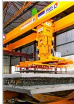
capacity of 5 tons operates on the existing crane as well, weight saving had maximum priority. The design engineers succeeded in reducing the maximum wheel loads by restricting the traveling path of the trolley. In addition, Brunnhuber strengthened the crane's frame around the lifting beam crane; the trolley frame is based on wheel blocks from Stahl CraneSystems. For the limiting gear, a tackle type SH 40, a separate, two-groove cable drum without lateral movement, was constructed.
