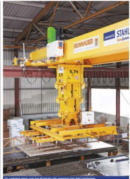
The customised stacker crane from Brunnhuber with components from Stahl CraneSystems.
