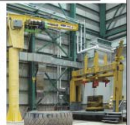
A slaving crane for changing tyres, the SH wire rope hoist can lift up to six.
