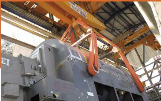
01 The crane trolley of the double-girder overhead travelling crane is equipped with a 180-tonne winch and a 25-tonne wire rope hoist
