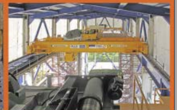
02 As "smaller" auxiliary hoists, both cranes have a 25-tonne wire rope hoist
