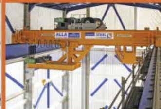
01 The crane trolley of the double-girder overhead travelling crane is equipped with a 180-tonne winch and a 25-tonne wire rope hoist
