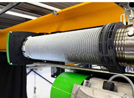
Image 3. The improved rope guide protects the rope, prevents it from being overwound, reduces maintenance requirements thanks to simple installation, as well as ensuring reliability and safety.
