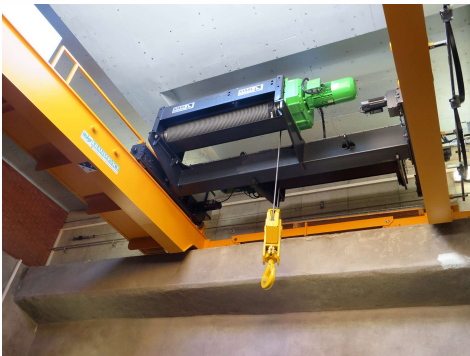
Wire rope hoist from STAHL CraneSystems for a maximum lifting height of 102 m and load capacities up to 16 t
