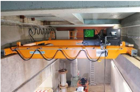
Double-girder bridge crane with twin hoists and continuous load monitoring
