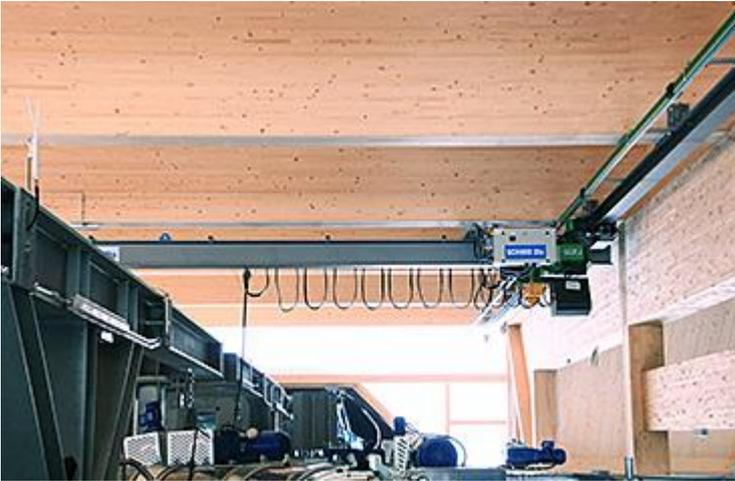
The hoist (max. lifting height 19 m) of the 2-ton crane in the middle station should have as much space as possible for the maintenance areas. Therefore, a STK 50 chain hoist with extra-short headroom trolley and integrated special chain box was chosen.
