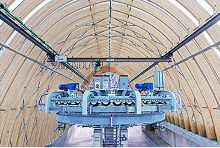
The single-girder suspension crane in the valley station with a load capacity of 2 tons and a lifting height of 8.5 m, of which the approximately 36-metre-long crane track was suspended on a total of 39 wooden trusses.
