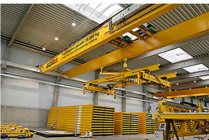
The complete crane including load attachment device is controlled by radio remote control.
