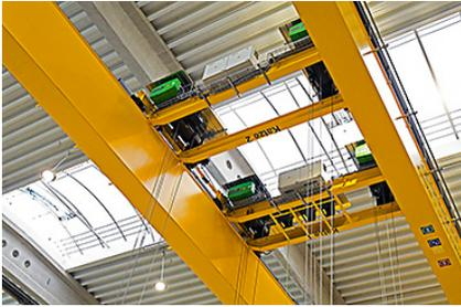
STAHL CraneSystems supplied 4 SH wire rope hoists, SR wheel blocks with radio-controlled travel drives for the construction of the two crabs, coupled LT endcarriages, the travel drives for the crane bridge and the complete control and commissioning.
