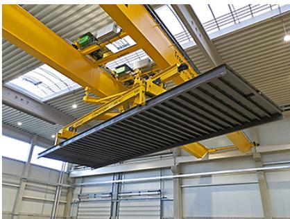
The crane picks up the pallets from the production area in longitudinal direction to the hall, turns them by 90° with the help of an automatic positioning feature ...
