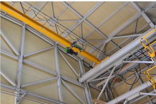
Single girder overhead travelling crane in the third-largest fertiliser factory in the world.
