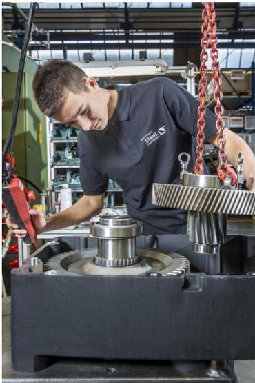
The apprentice Selim Benderdour assembling the gearbox for a hoist.
