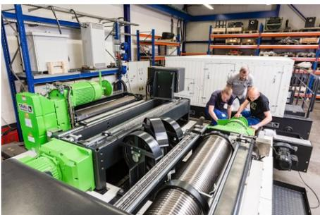
Special order for a Russian gas-to-liquids plant. These hoists must function in outdoor temperatures as low as  $-50\text{ }^{\circ}\text{C}$ .
