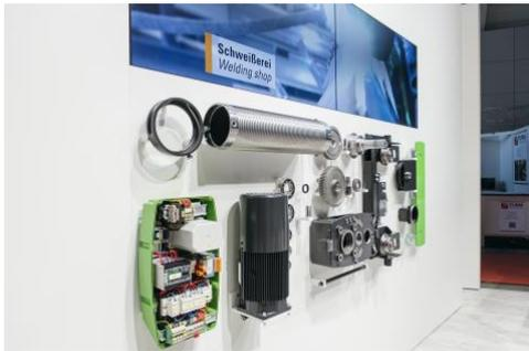
At the stand visitors could inspect the individual components of a wire rope hoist. Every single part is manufactured in STAHL CraneSystems' plant in Künzelsau, as shown in a video clip.
