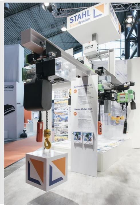
STAHL CraneSystems presents the new ST 50 chain hoist with a lifting capacity of 2,500 to 5,000 kg at LogiMAT in Stuttgart. The gearbox limit switches, brake and contactor control could be seen in the prototype through Plexiglas.
