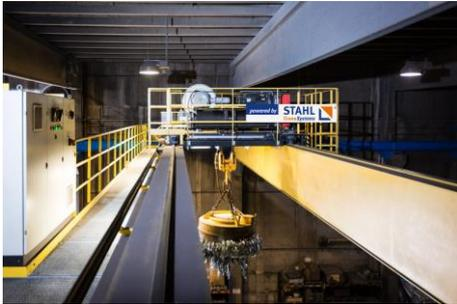
Thanks to the compact dimensions of the trolley and wire rope hoist, the new crane system could be integrated into the existing hall and still offer the required lifting height.
