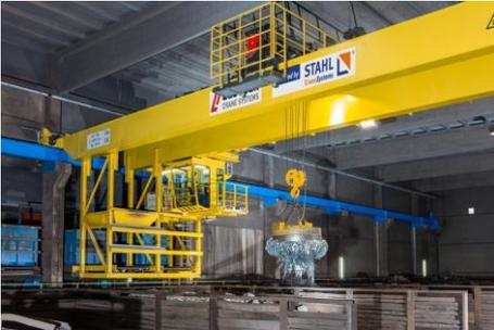
During charging, the portal crane drives through the hall of the raw material mixing plant to the storage bunkers at speeds of up to 63 m/min.
