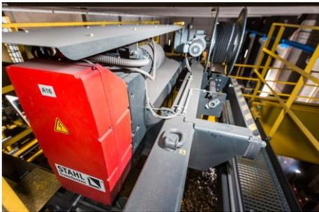
Powerful technology in the tightest of spaces: The SH wire rope hoist in the typical red of Austrian CraneSystems is designed for especially high loads and is the optimum choice for demanding processes.
