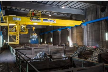
Metallic bulk materials of different grades and composition are stored in 25 separate bunkers – the ingredients for new castings.
