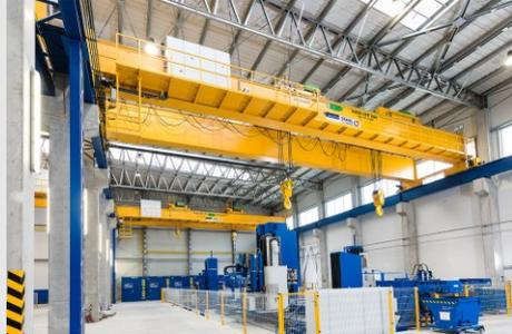
Four of these double girder overhead travelling cranes work in the new factory building of VVE, a slovakian manufacturer of hydroelectric power plants. The structural engineering calculation necessitated additional supporting pillars under the crane runway and demanding safety precautions by the crane technology.
