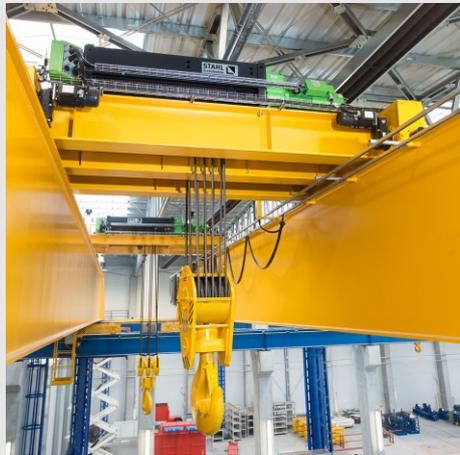
Heavy duty machinery with compact dimensions: the ASF 7 ZW wire rope hoist from STAHL CraneSystems lifts up to 125 t. An ASF 7 wire rope hoist with S.W.L. of 55 t serves as auxiliary hoist on this crane.
