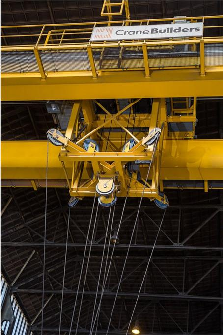
Sophisticated technology from the Netherlands: the rigid rope bracing mounted under the crab can lift the grab vertically and without rotating. Even diagonal pull does not cause increased stress or premature wear on the wire rope hoists.
