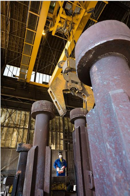
The crane operator controls by radio the massive grab with which the cylinders of fresh-cast steel are lifted.
