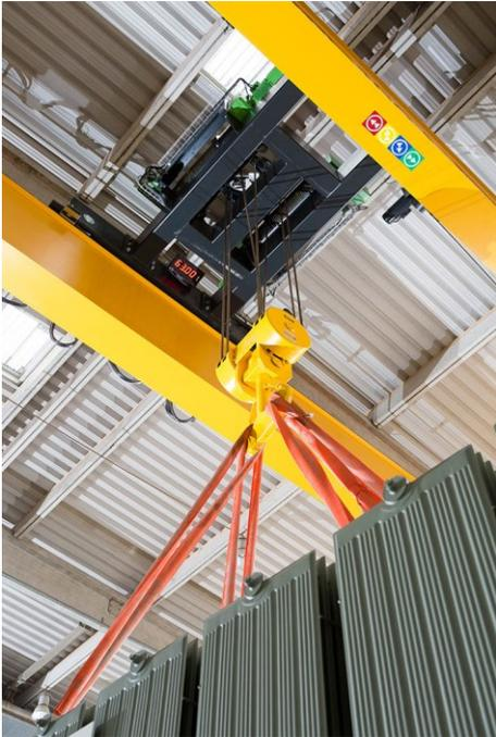
The load is crosschecked by means of a load display.
