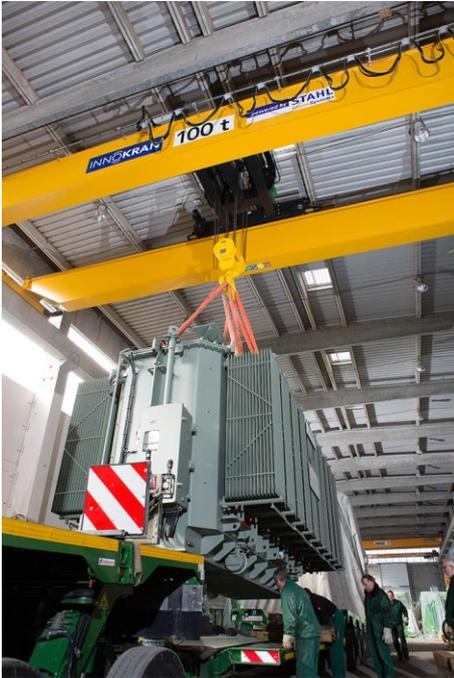
Heavy load: the new crane loads transformers weighing over 70 t onto a special-purpose vehicle.
