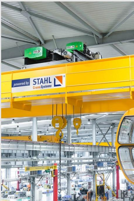
Many of the cranes operate with two hoists on the double rail crab – the larger wire rope hoist acts as main hoist, the faster, smaller wire rope hoist as auxiliary hoist.
