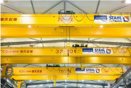
The crane with the highest capacity has one 75 t and one 20 t wire rope hoist.
