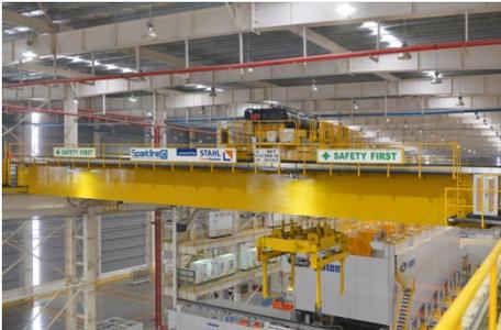
The heart of the crane systems are SHW 8 rope winches from STAHL CraneSystems. During production in Künzelsau they were equipped for particularly high speeds and operating with tool grabs.
