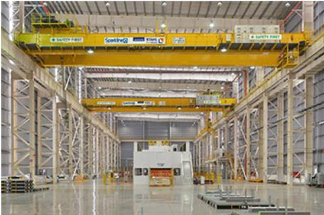
State of the art production at Ford India. Automatic process cranes with STAHL CraneSystems components are used for retooling the press and stamping lines.
