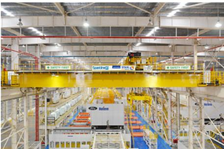
Fast tool change from the air: the cranes approach the desired tool position at a speed of up to 60 m/min, take up the tool and transport it to the designated storage area. Equipping the press with the next tool is also automatic.
