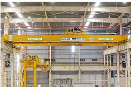
Operating on more than one level: effective collision protection is essential to prevent the bridge cranes and semi-portal cranes colliding.
