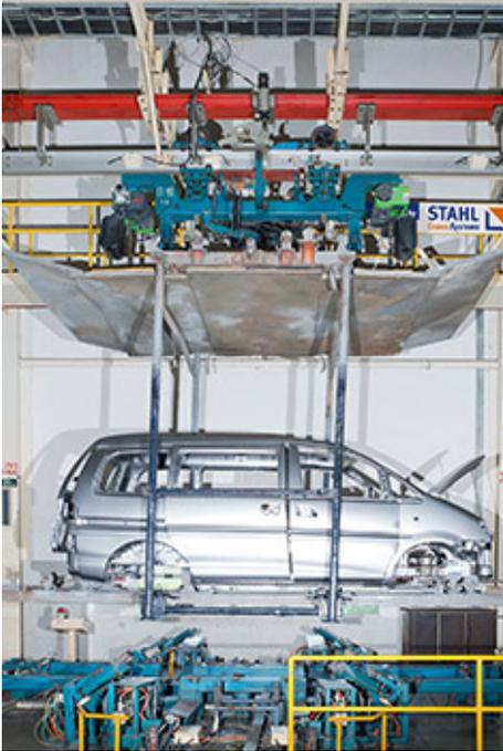
STAHL CraneSystems chain hoists have been in use at this automobile manufacturer since 2002. They help lower car bodies into paint tanks then lift them out again.
