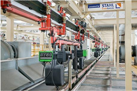
Pairs of ST 50 chain hoists lift whole car bodies. The Chinese company uses more than 150 ST and SC series chain hoists.
