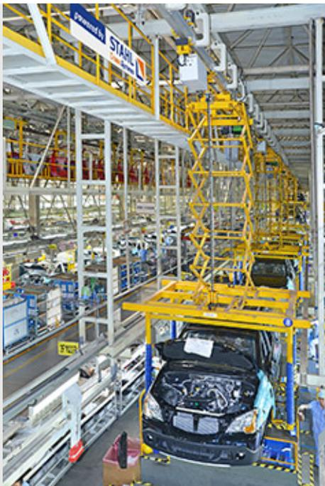
Nine STD 50 dual chain hoists are used in the final assembly of cars by a Chinese automobile manufacturer. Thanks to the STD's synchronous chain lead-offs the vehicles can be lifted perfectly level.
