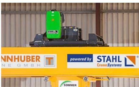
A low-wear solution for the rope drive was designed in close collaboration between Brunnhuber and STAHL CraneSystems. The basis of the customised solution is the field-proven SH 60 wire rope hoist which was manufactured with a double-groove rope drum for this crane.
