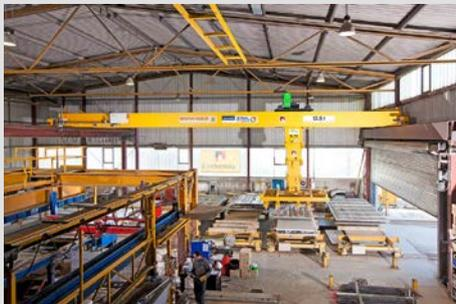
Reinforcements and intelligently limiting the crab's travel made it possible to use the existing crane runway.
