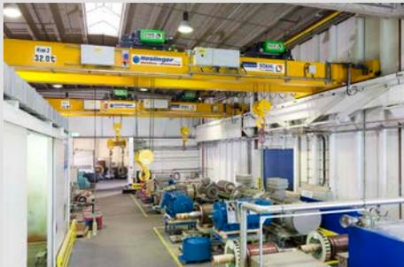
Each of the wire rope hoists can lift 32 tonnes, each crane is designed for 32 tonnes and the crane runway between the pillars is also designed for 32 tonnes. Position detection and load measurement and evaluation in a Siemens S7 control guarantee safety.
