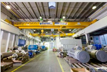
SIEMENS manufactures electric motors in its Ruhstorf plant. The crane system was upgraded from 2 x 16 to 2 x 32 tonnes S.W.L. in order to be able to transport the increasingly large and heavy motors.
