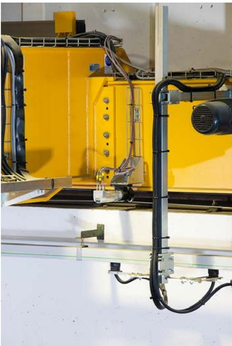
High-tech on the crane: position detection by means of drive belt (shown centre) and fail-safe data transmission.
