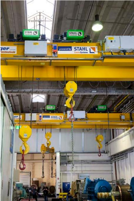
The wall in the background can be swivelled back so that the cranes can move into the neighbouring aisle to load the motors onto lorries.
