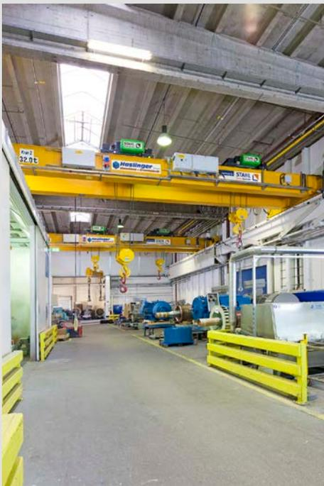
Two crane bridges, four wire rope hoists, one customised control: Haslinger's crane system is anything but standard. On the left of the photo: the paint shop.
