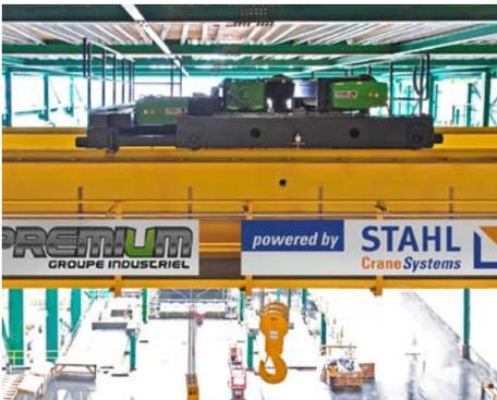
Powerhouse times two: the twin design AS 7 ZW stands for great height of lift, high lifting speed and a lifting capacity of up to 120 t while requiring little space. This twin hoist can lift up to 70 tonnes.
