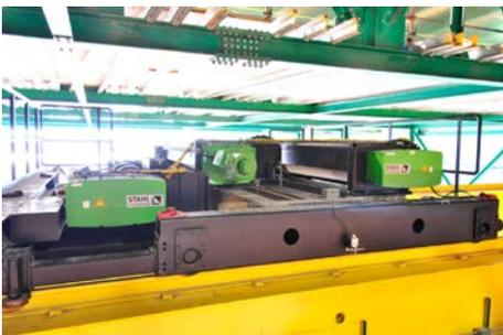
The SH wire rope hoist with a lifting capacity of 15 t mounted at the side comes into use for lifting lighter loads.
