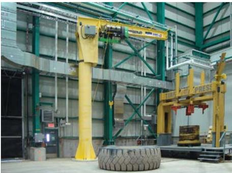
A slewing crane for changing tyres: the SH wire rope hoist can lift up to 10 t.
