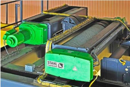
One of the advantages of this design: the ropes of the coupled AS 7 hoists run over a return sheave so that true vertical lift is possible.
