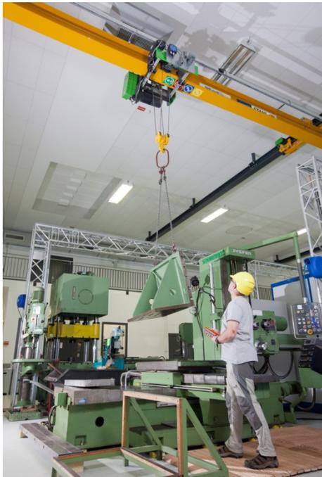
The suspension crane is used in the PTB's scientific apparatus-building department for transporting heavy tools and machinery parts.
