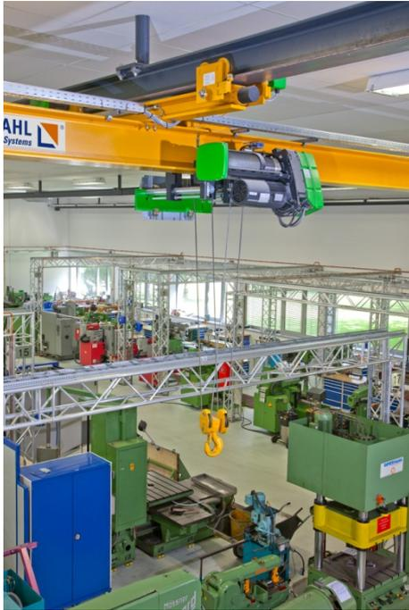
Crane technology for demanding crane builders: STAHL CraneSystems supplied suspension crane endcarriages, travel drives and of course the wire rope hoist for this customised crane.
