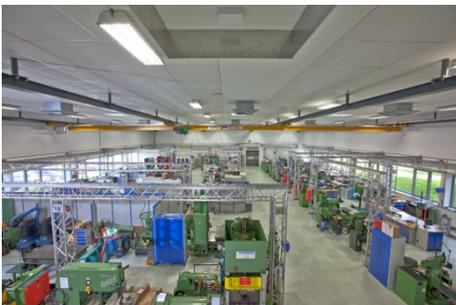
Thanks to the four-section suspension it was possible to manufacture the 26 m long crane bridge from sectional beams and ensure lower headroom.
