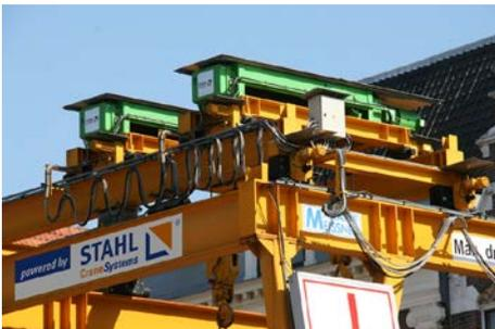
The connection of two hoists permits hoisting speeds of 15 m/min under full load or 21 m/min with an empty container, equivalent to the 15 load cycles per hour calculated by construction company Max Bögl.
