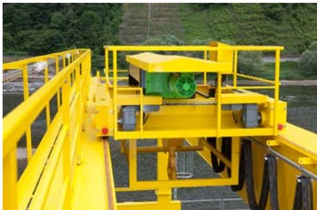
The AS 7 wire rope hoist from STAHL CraneSystems is protected by a roof. The crab is easily accessible from a maintenance bridge.
