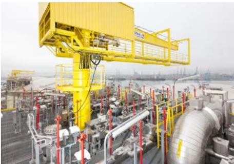
The casing protects the hoist from wind and weather.
