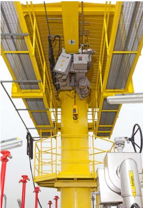
STAHL CraneSystems' off-standard LNG hoists are certified in compliance with ATEX and thus approved for use in hazardous areas.
