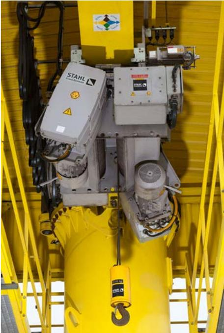
The redundant design ensures safe operation even if one of the hoists should fail.
