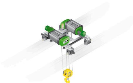
On the AS 7, motor, gear and rope drum are arranged in line. This central gear concept permits high outputs and loads. As a twin hoist the AS 7 achieves higher hoisting speeds and greater heights of lift, and safe working loads up to 125 tonnes.
