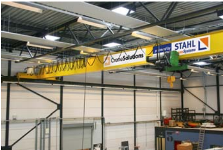
Picture 2: Single girder overhead travelling crane with wire rope hoist SH3005-25-4/1
