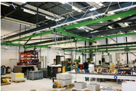
Picture 4: KT2000 Small Crane System with S.W.L. from 250 kg to 500kg, runway length 19 meters
